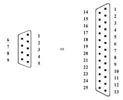
Depending on the pin assignment of the serial (RS232) connector, computers are classified into two categories:
