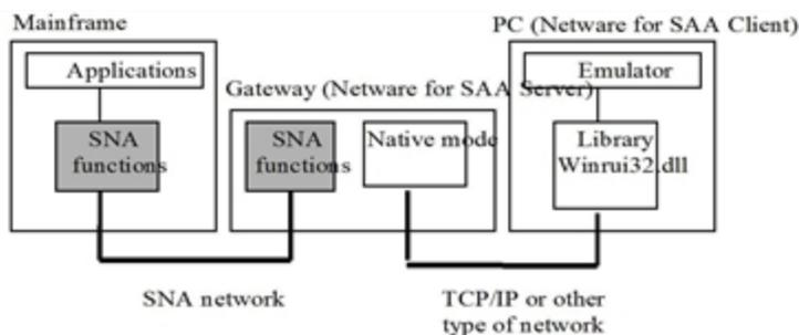
To use Esker's IBM 3270 emulator via a Netware for SAA gateway in native mode, you must first install the **Novell Netware client** on your PC (which includes **Winrui32.dll**) as well as the **IntranetWare for SAA client** from **Novell**.
