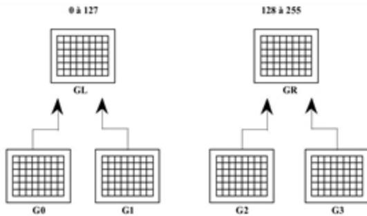
By default, one of the tables G0, G1, G2, or G3 is loaded into GL and GR. GL represents all the characters from 0 through 127, and GR, the characters from 128 through 255.
