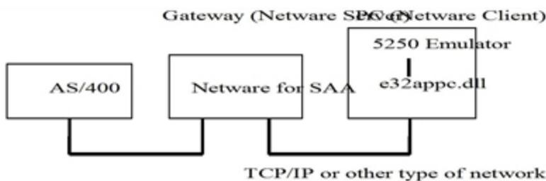
The PC running the emulator must have **Novell's Netware** client (which comprises API **e32appc.dll**) as well as **Novell's Intranetware for SAA** client.
