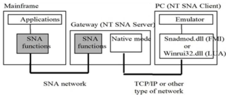
To use Esker's 3270 IBM emulator in native mode with a Microsoft SNA Server gateway, you must first install the client part of SNA Server on the PC (SNA Server Client, version 3.0) supplied with Microsoft® **BackOffice**®. See Microsoft's documentation for installation details.
